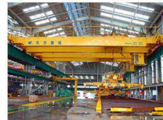
QCL 型旋转挂梁桥式起重机 QCL overhead crane with rotary carrier-beam
