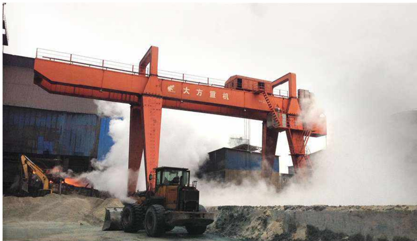
唐山东海特钢集团室外干渣作业区使用的大方重机双梁龙门产品。 Double girder gantry crane made by DA Fang Heavy machinery co.,ltd used on outdoor dry slag operation area in Tangshan Donghai special steel group
