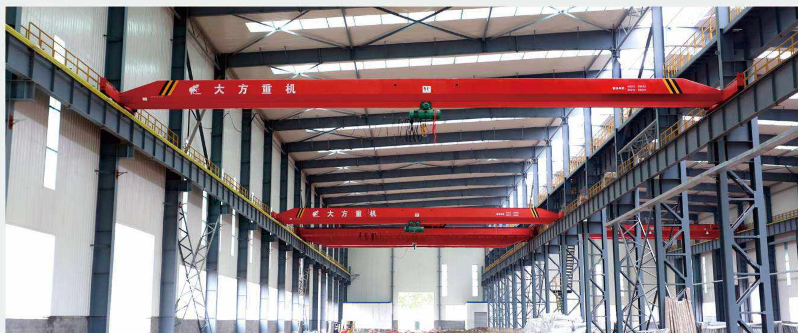
LD 型电动单梁起重机 LD model electric single girder crane
