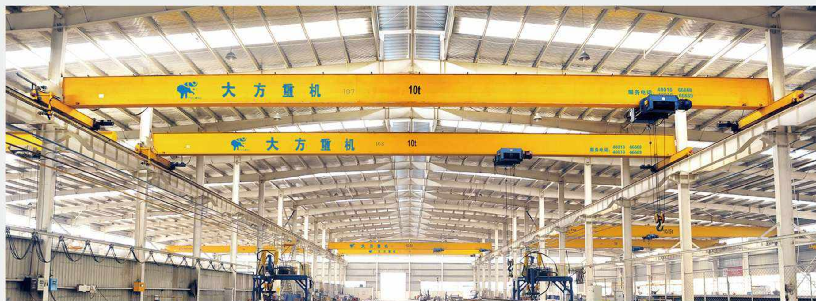
HD 型欧标电动单梁起重机 HD model electric single girder crane
