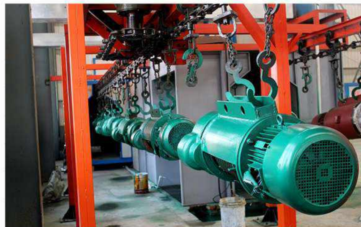
电动葫芦烤漆线 electric hoist painting line
