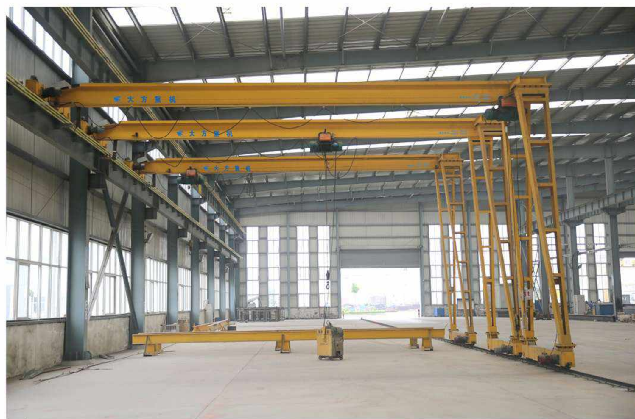
MHB 型电动葫芦半门式起重机 MHB type electric hoist gantry crane
