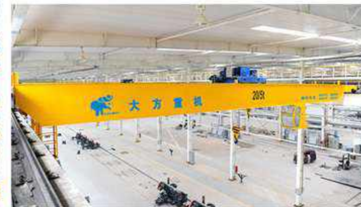
欧标葫芦双梁桥式起重机 light duty hoist double girder overhead crane
