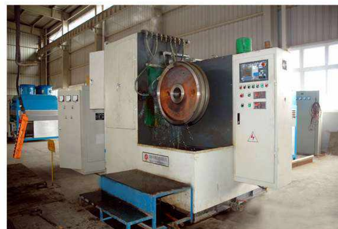
车轮数控淬火机 wheel NC hardening machine
