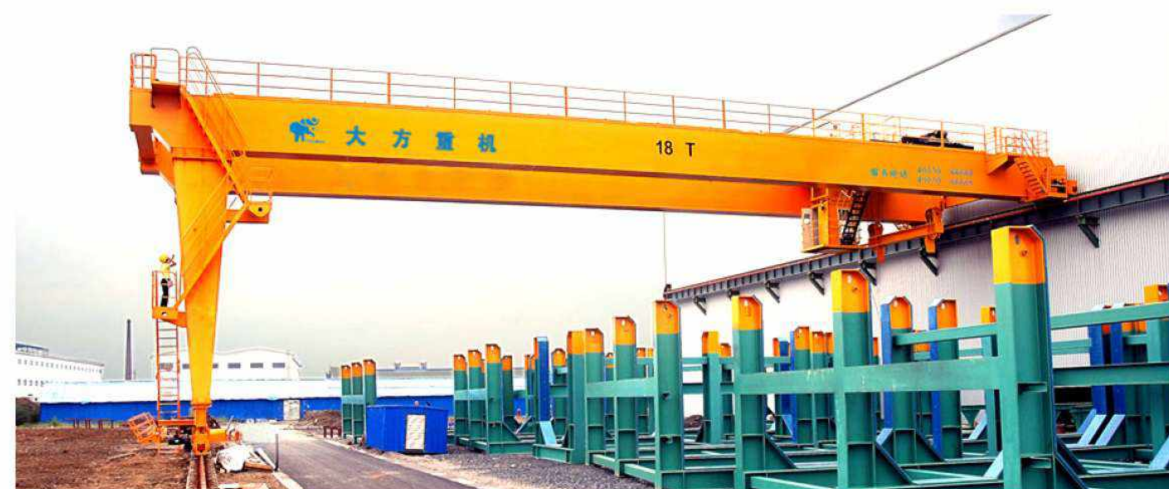
MGB 型通用半门式起重机 MGB type general-purpose gantry crane
