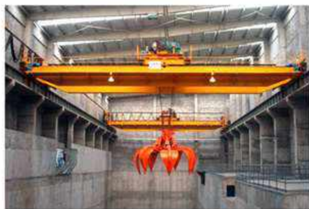
QZ 型抓斗桥式起重机 QZ overhead crane with grab
