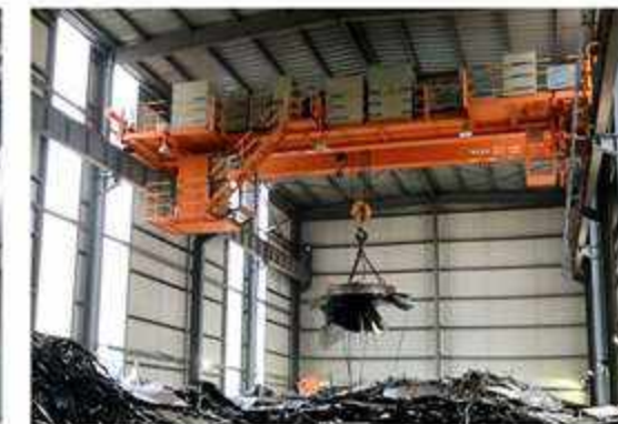
QC 型电磁桥式起重机 QC electromagnetic overhead crane
