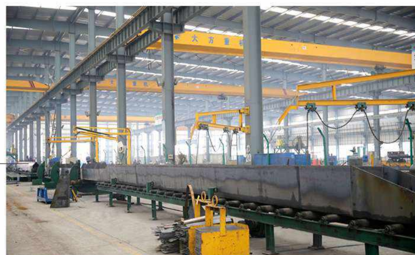
主梁组对 main girder assembly
