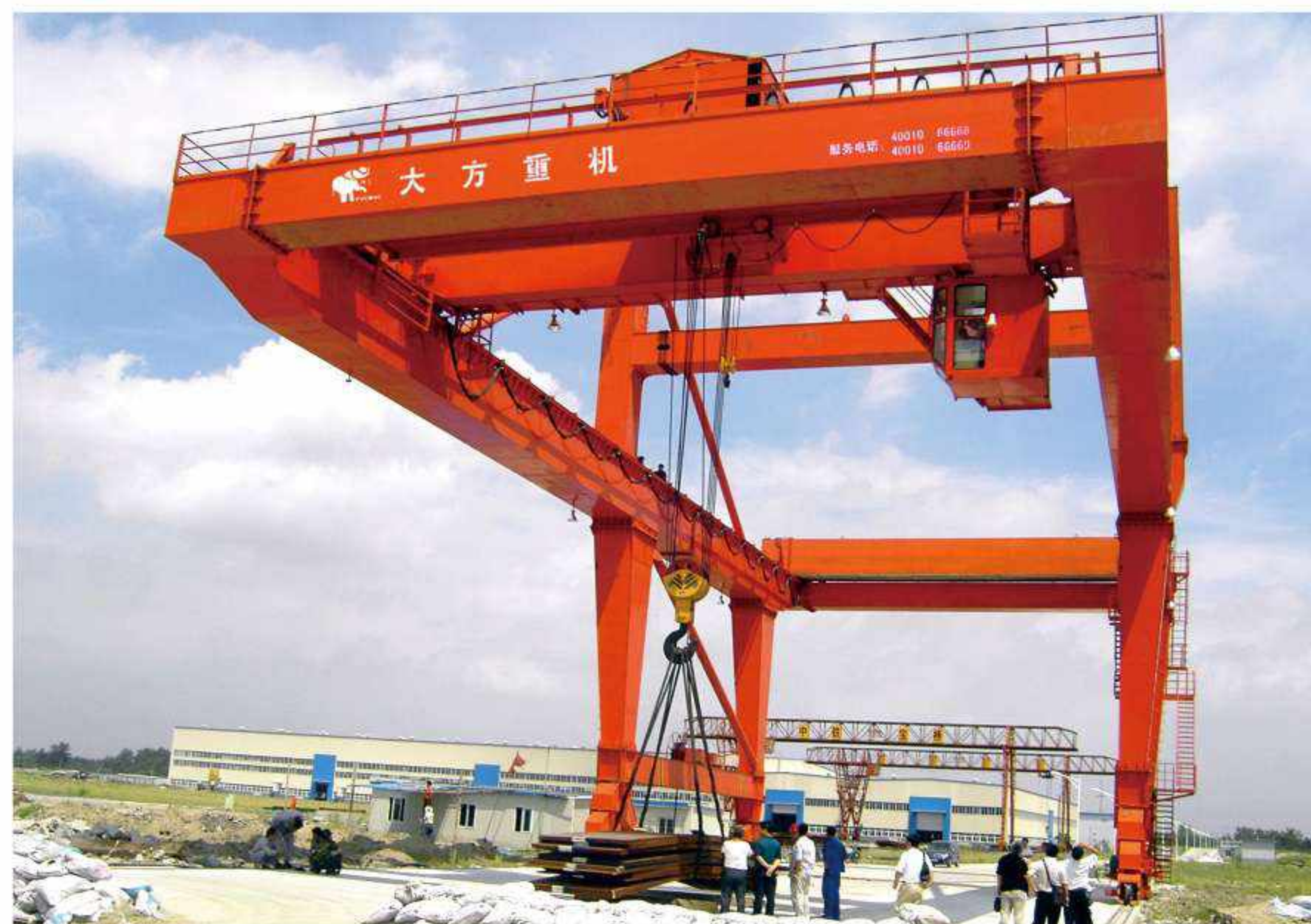
装卸桥 loading bridge
