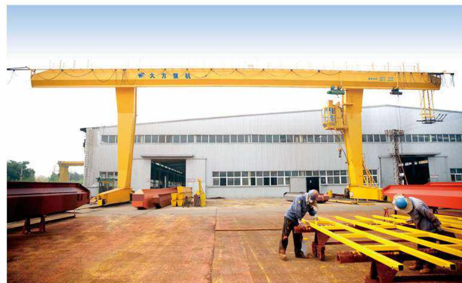
L 型电动葫芦门式起重机 L type electric hoist gantry crane
