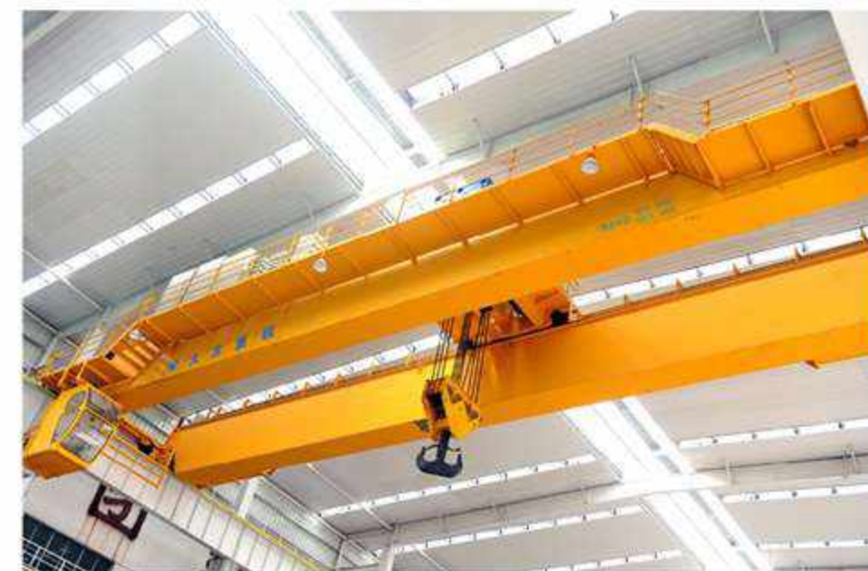
QCL 型旋转挂梁桥式起重机 QCL overhead crane with rotary carrier-beam
